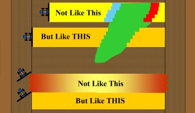
Immediate Nozzle "ON and "OFF" By Section or Entire Boom
