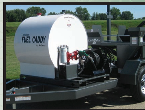
Optional FC300SS, 300 Gallon Fuel Caddy Allows Filling Fuel And Seed At The Same Time Fuel Caddy Can Easily Be Unbolted And Placed In A Pickup During Harvest
